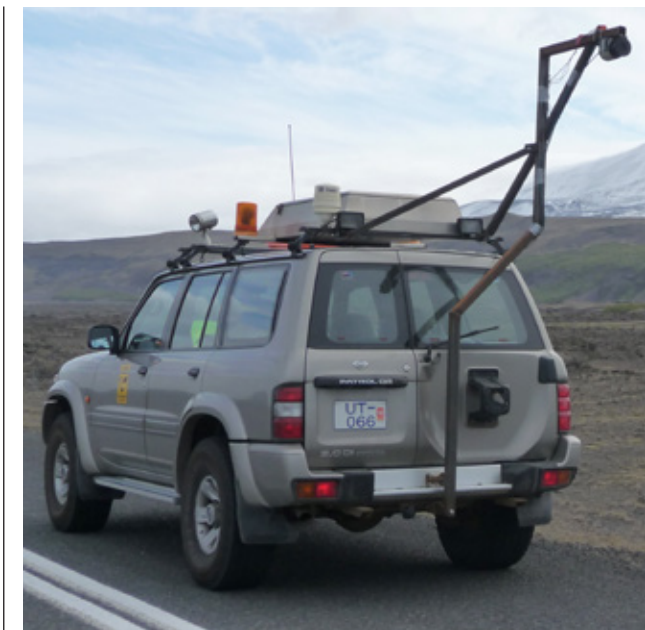
ICERA survey vehicle in Iceland equipped with laser scanner for road speed drainage surveys (photo: Seppo Tuisku)
