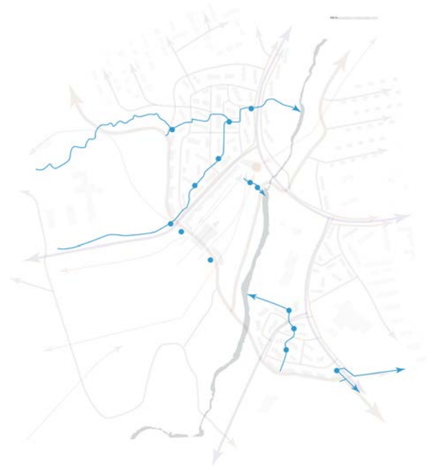
Channels and detention ponds for excess thaw water.
