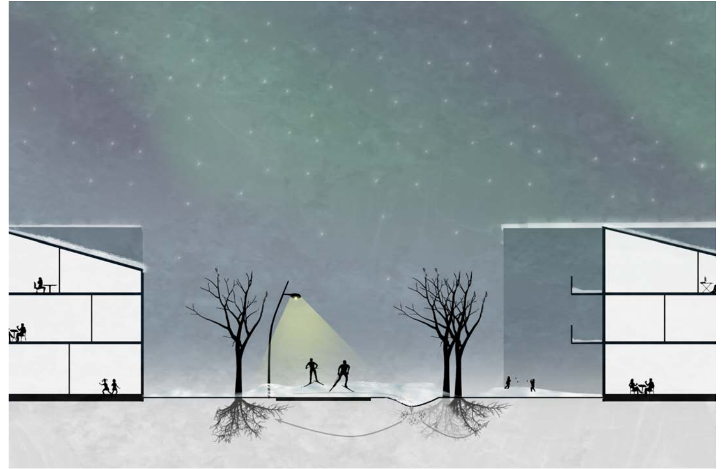
Skiswale path space doubles as a bioswale allowing natural filtration, providing water for the surrounding vegetation, and channeling excess thaw water towards detention ponds.
