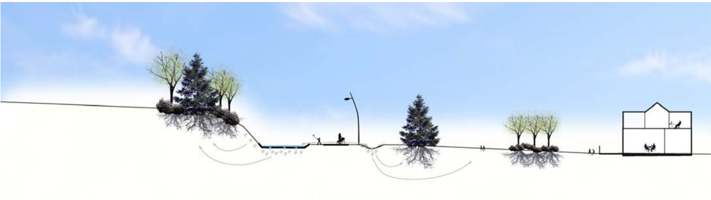
The Ribbon in summer-mode where the snow-storage basin becomes a storm-water basin. The Skiswale path is a regular path for pedestrians, bikers and a space for play.
