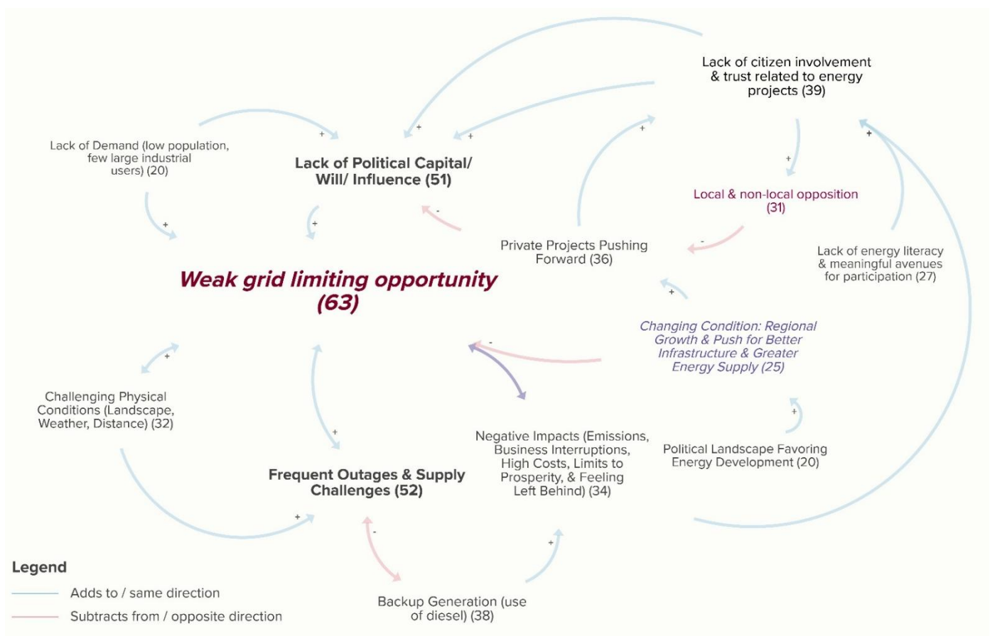
Figure 15. Causal Loop Diagram of the energy system in the Westfjords with components sized proportionally to how frequently participants observed them
